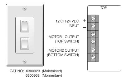
The Decorator DC switches are SPDT, center off, maintained or momentary switches. They can be used with DC motors, models LT28, LV35 and V26.
