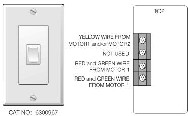
This switch is intended for use with either 1 or 2 DR1000 Drapery Motors. The UP direction operates Motor1 and the DOWN direction operates Motor2. Each switch press will sequence the motor through open, stop, close, stop. To operate more than one DR1000 as a group, please contact Somfy Systems customer service.
