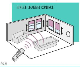
A 5 channel transmitter can control up to 5 specific groups of window coverings
